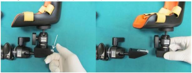
Tighten the screw of the quick release adaptor with 2.6Nm by using a Torque wrench with a Phillips PH2 Bit.
