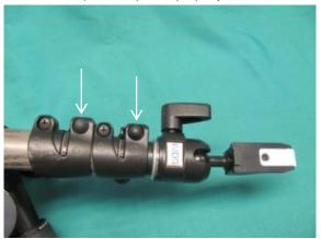
In case the spindle cap is loose it has to be fixated by using e.g. Loctite 326-50 ML bonding application.
