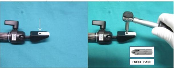
Do not remove the bolts of the friction mechanism by completely disassembling them. These bolts consist of 2 parts that can easily be lost. As a consequence the clamp function will not work anymore.
