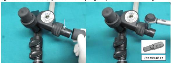
3 The cap of the clamping socket has to be fixated by using e.g. Loctite 326-50 ML bonding application.
