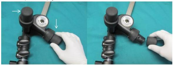
2 Tighten the screw of the clamping sockets with **6Nm** by using a Torque Wrench with a 3mm Hexagon Bit.
